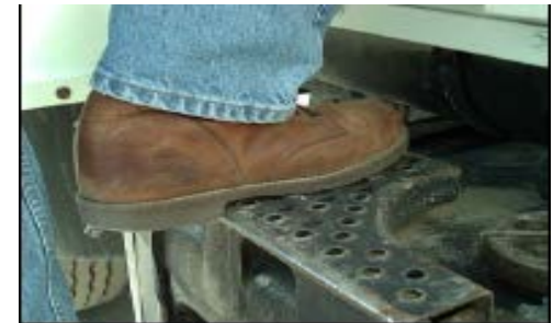
Facing the truck means better foot contact with steps and platforms.
